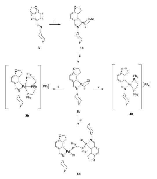
Scheme 3. (i) Pd(AcO)<sub>2</sub>, toluene; (ii) NaCl, acetone/water; (iii) triphos (1:2), NH<sub>4</sub>PF<sub>6</sub>, acetone/water; (iv) dppm (1:2), NH<sub>4</sub>PF<sub>6</sub>, acetone/water; (v) dppm (1:1), acetone/water.
