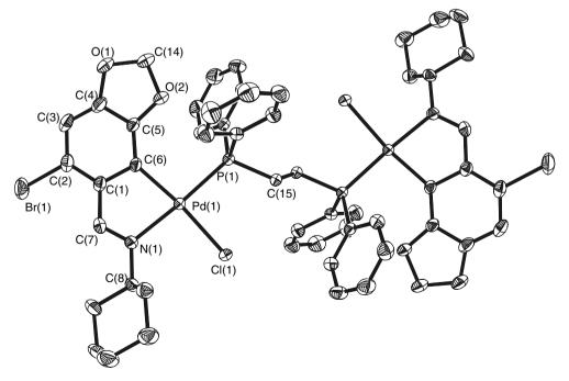
Fig. 6. Molecular structure of [{Pd[2-Br-4,5-(OCH<sub>2</sub>O)C<sub>6</sub>HC(H)=N(Cy)-C6,N]}<sub>2</sub>{ $\mu$ -Ph<sub>2</sub>PC(H)=C(H)PPh<sub>2</sub>}](**5a**), with labelling scheme. Hydrogen atoms have been omitted for clarity.
